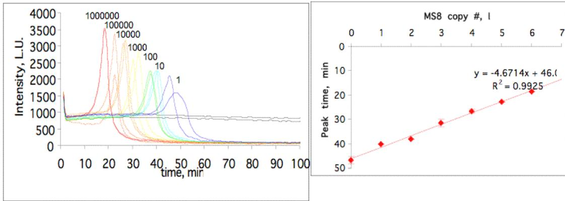
Figure 9. Example of detection of MS8 within 20-50 minutes, with sensitivity to single copy. Left: raw BART outputs showing light intensity against time. **Note the duplicate negative controls show a flat line with residual signal maintained.** Right: plot of log concentration against time to peak.
