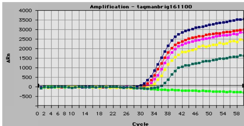
Figure 1. Amplification plot from an Applied Biosystems 7700 Real-Time PCR system. Graph shows the change in fluorescence signal plotted against cycle number. The amplification plot reflects the generation of the reporter dye during amplification and is related directly to the formation of PCR products. Coloured lines represent different standards of known target analyte concentration.
