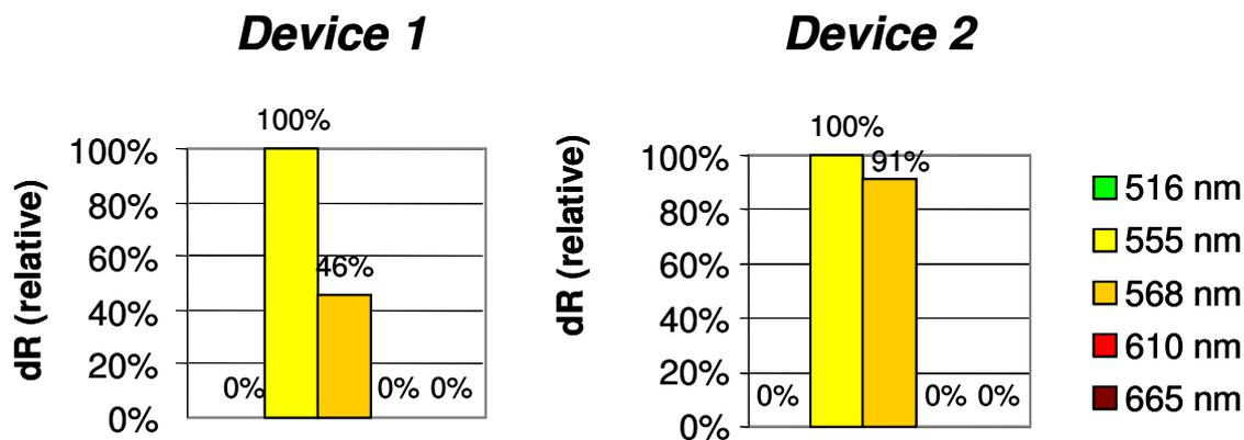
Figure 17. Cross-talk effect of HEX dye (yellow) to the neighbour channels FAM (green), Cy3 (orange), ROX (red), Cy5 (dark red) on two different qPCR platforms.
