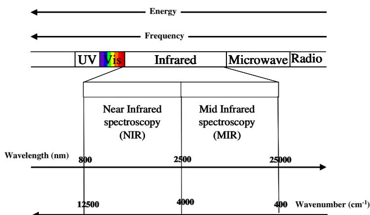
**Figure 1:** NIR and MIR spectroscopy in the electromagnetic spectrum
