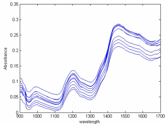
**Figure 9:** Mean NIR spectra obtained for each of the 10 grains represented in Figure 8a
