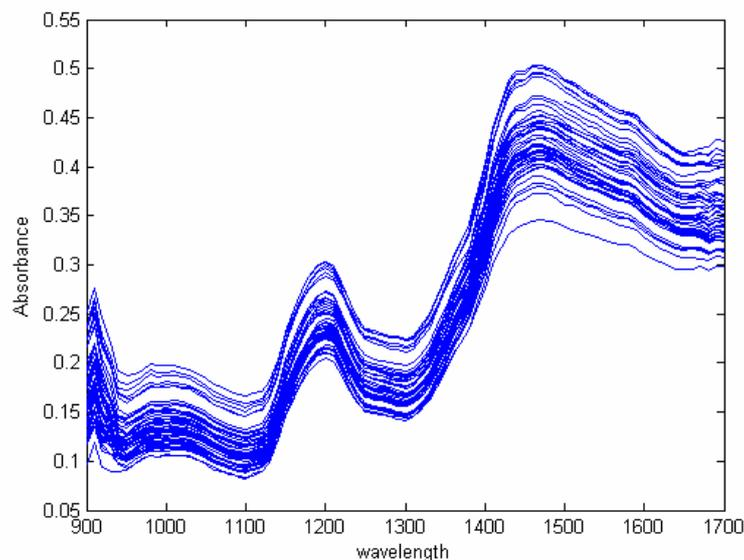
**Figure 3:** NIR spectra of soybean kernels obtained with the NIR camera. Each spectrum is the mean of the spectra from the pixels area covered by the grain.
