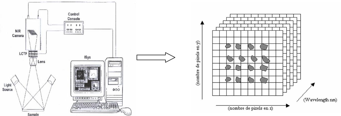
**Figure 2:** NIR imaging system and spectral volume obtained with it.
