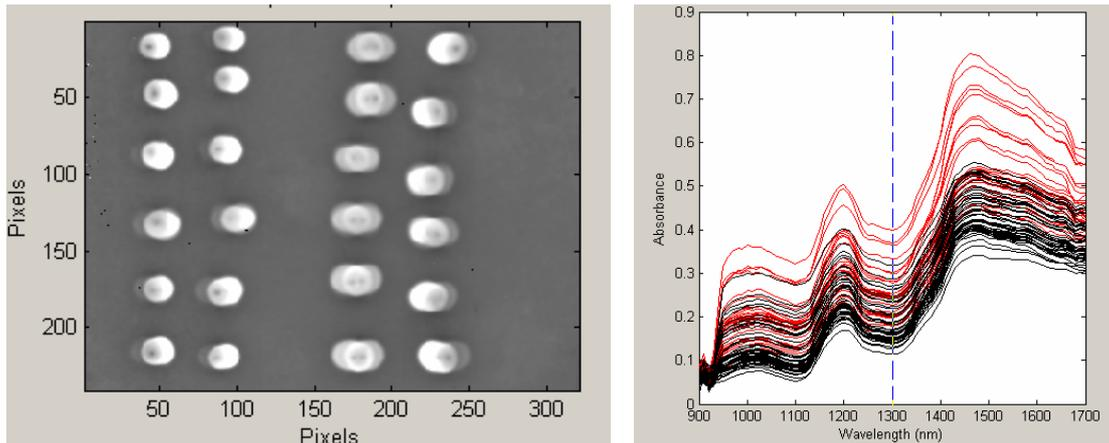
**Figure 5:** a) Example of a NIR image of soybean kernels obtained with the NIR camera and b) the whole mean spectra for dataset 1. Black spectra correspond to non GM samples and red spectra to GM samples.
